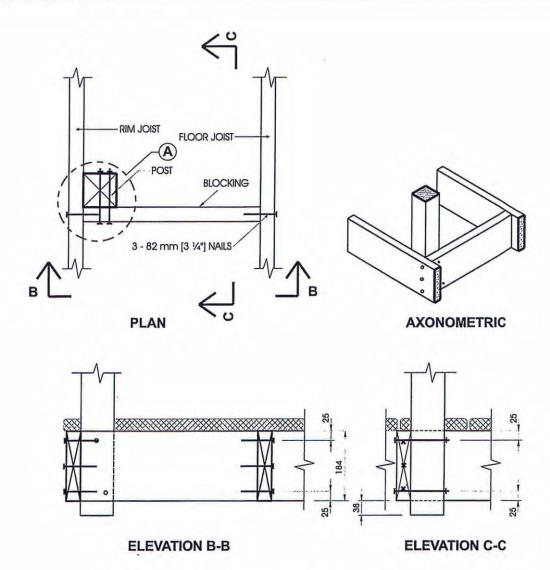
**Detail EB-6** Exterior Connection: Post Fastened to Floor, Guard Parallel to Floor Joists
