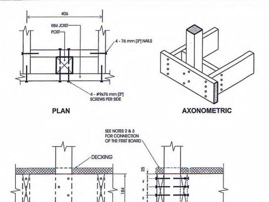
**Detail EB-2 Exterior Connection: Post Screwed to Rim Joist**
