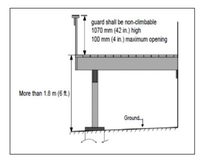
The OBC requires that guards be installed on walking surfaces on each side that is not protected by a wall where [9.8.8.1(1)]:
