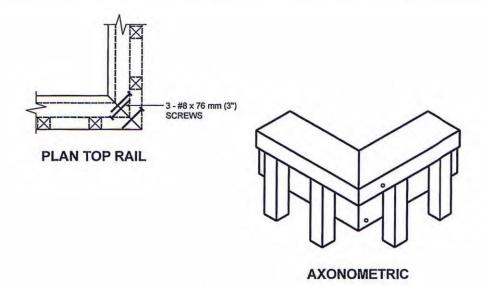
ONE FASTENER IN HORIZONTALLY ORIENTATED PORTION OF TOP RAIL AND TWO IN VERTICALLY ORIENTATED PORTION.
