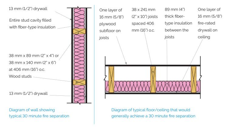
Good-to-Know: A wall built to meet the Building Code's fire separation requirements will help to reduce noise between units.
